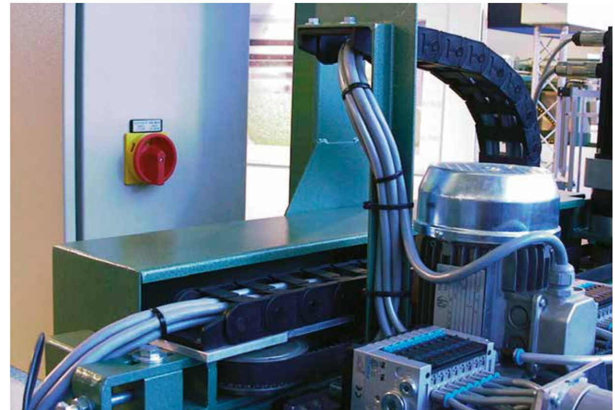
chainflex® CF140.UL in the feeder automation. e-chain®: easychain®
