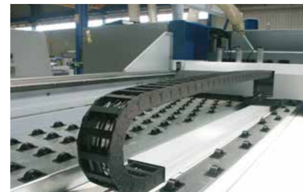
chainflex® CF130.UL for woodworking. e-chain®: E4/light
